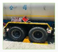
Inspection to confirm wheel chock placement behind tank truck wheels
