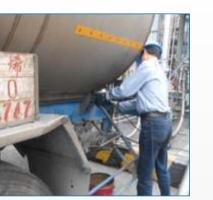
Confirmation of proper connection of ground wires
