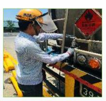
Confirmation of ground wire connection for tank trucks
