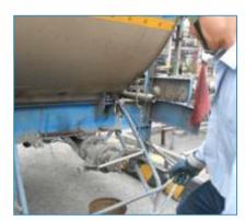
Confirmation of proper connection of high-pressure tubes
