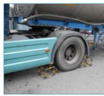
Inspection of proper placement of wheel chocks
