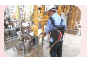
VOCs testing (1) VOCs testing (2) VOCs testing (3)
