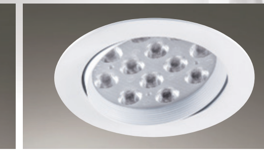
嵌入孔 ø115mm AL2509C 3000 W140mm H65mm 附高亮度原裝進口 OSRAM LED 15w AC100V-240V 3000K / 流明1800Lm 鋁
