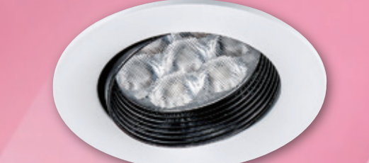
AL25109 2470 W90mm H55mm 附高亮度原裝進口 OSRAM LED 11w AC100V-240V 3000K / 流明1200Lm 鋁
