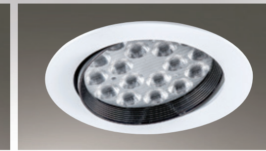
嵌入孔 ø115mm AL2509B 3340 W140mm H70mm 附高亮度原裝進口 OSRAM LED 22w AC100V-240V 3000K / 流明2250Lm 鋁
