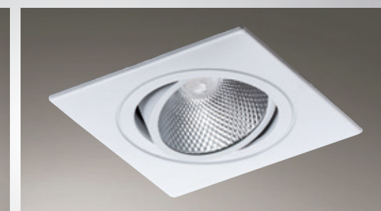
嵌入孔 ø75mm AL25083 2000 W93mm H55mm 附高亮度原裝進口 CREE LED 7.5w AC100V-240V / 3000K 鋁
