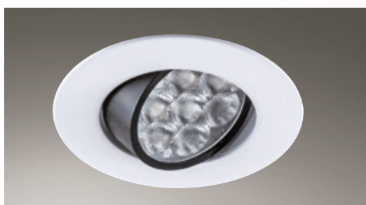
AL25104 2270 W84mm H50mm 附高亮度原裝進口 OSRAM LED 11w AC100V-240V 3000K / 流明1200Lm 鋁
