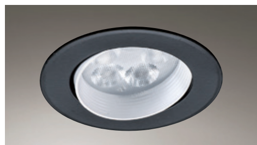
AL25102 2070 W84mm H45mm 附高亮度原裝進口 OSRAM LED 8w AC100V-240V 3000K / 流明900Lm 鋁
