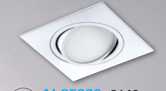
嵌入孔 ø75mm AL25089 2140 L93mm W93mm H55mm 附高亮度原裝進口 CREE LED 7.5w AC100V-240V / 3000K 鋁、散光
