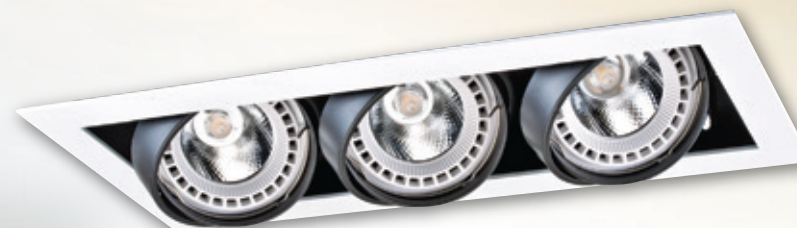
嵌入孔 465x170 mm AL25017 10000 L495mm W205mm H85mm 附COB LED 12wx3、黃光 鋁框、科銳晶片
