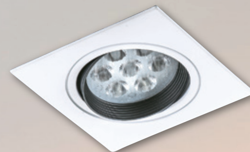
AL25111 3000 L121mm W121mm H75mm 附高亮度原裝進口 OSRAM LED 11w AC100V-240V (台灣電子) 3000K / 流明1200Lm 鋁
