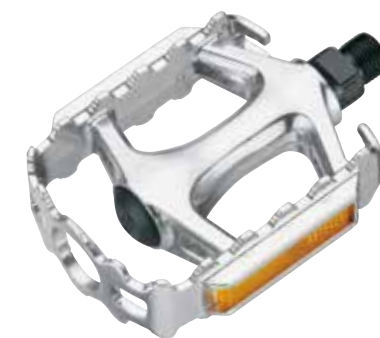
NWL-106 SIZE 105x82x24mm WEIGHT 423g/PR BODY Burnished silver alloy AXLE Boron / Cr-Mo BEARING Loose balls REFLECTOR Included
