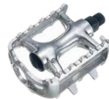
NWL-936 SIZE 105x72x24mm WEIGHT 430g/PR BODY Burnished silver alloy AXLE Boron / Cr-Mo BEARING Loose balls
