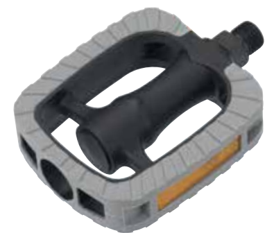
NW-357 SIZE 107.5x82x25.5mm WEIGHT 343g/PR BODY One piece PP body with TPR rubber AXLE Boron / Cr-Mo BEARING Loose balls REFLECTOR Included
