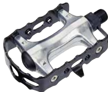
NWL-90R SIZE 105x63x25mm WEIGHT 447g/PR BODY Burnished silver alloy body CAGE Steel / Alloy AXLE Boron / Cr-Mo BEARING Loose balls TOE CLIP Available TOE STRAP Available
