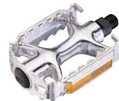
NWL-979 SIZE 105x78x24mm WEIGHT 480g/PR BODY Burnished silver alloy AXLE Boron / Cr-Mo BEARING Loose balls REFLECTOR Included
