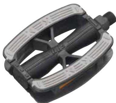
NW-353 SIZE 100x80x25mm WEIGHT 416g/PR BODY One piece PP body with TPR rubber AXLE Boron / Cr-Mo BEARING Loose balls REFLECTOR Included
