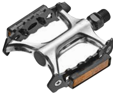
NWL-452L SIZE 117x82x21mm WEIGHT 300g/PR BODY Burnished silver alloy body CAGE Steel / Alloy AXLE Boron / Cr-Mo BEARING Loose balls
