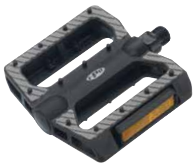
NW-420 SIZE 107x102x25mm WEIGHT 352g/PR BODY One piece PP body with TPR rubber AXLE Boron / Cr-Mo BEARING Loose balls
