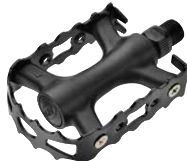
NW-499 SIZE 109x63x22.5mm WEIGHT Alloy cage 320g/PR Steel cage 385g/PR BODY One piece PP body CAGE Steel / Alloy AXLE Boron / Cr-Mo BEARING Loose balls
