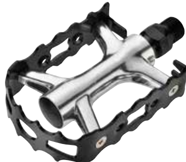
NWL-499 SIZE 109x63x20mm WEIGHT Alloy cage 340g/PR Steel cage 395g/PR BODY Burnished silver alloy body CAGE Steel / Alloy AXLE Boron / Cr-Mo BEARING Loose balls
