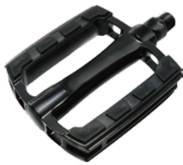
NWL-609 NEW SIZE 91.2x84.6x21.7mm WEIGHT 427g/PR BODY One piece PP body with TPR rubber AXLE Boron / Cr-Mo BEARING Loose balls REFLECTOR Included
