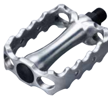
NWL-399N SIZE 105x73.7x27mm WEIGHT 436g/PR BODY Burnished silver alloy AXLE Boron / Cr-Mo BEARING Loose balls
