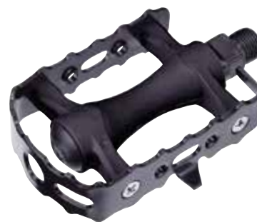
NW-90R SIZE 106x62x25mm WEIGHT 420g/PR BODY One piece PP body CAGE Steel / Alloy AXLE Boron / Cr-Mo BEARING Loose balls TOE CLIP Available TOE STRAP Available
