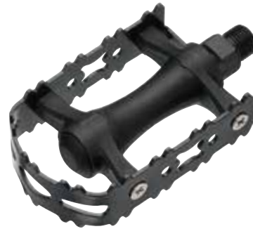
NW-96K SIZE 105x62x25mm WEIGHT 288g/PR BODY One piece PP body CAGE Steel / Alloy AXLE Boron / Cr-Mo BEARING Loose balls
