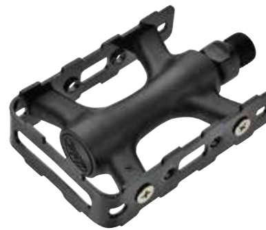
NW-517 SIZE 96.4x62x24mm WEIGHT Alloy cage 264g/PR Steel cage 334g/PR BODY One piece PP body CAGE Steel / Alloy AXLE Boron / Cr-Mo BEARING Loose balls
