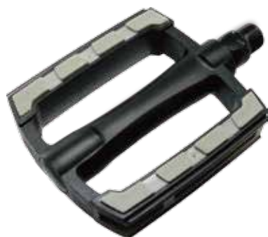
NW-609 NEW SIZE 112.6x84x27.3mm WEIGHT 300g/PR BODY One piece PP body with TPR rubber AXLE Boron / Cr-Mo BEARING Loose balls REFLECTOR Included
