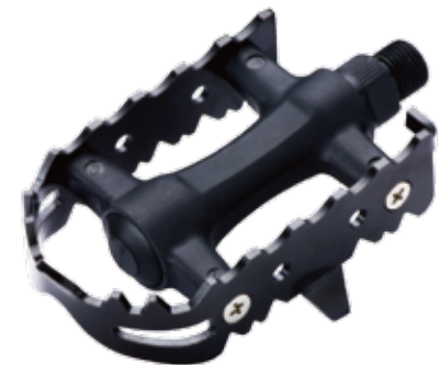
NW-93K SIZE 110x62.5x25mm WEIGHT 415g/PR BODY One piece PP body CAGE Steel AXLE Boron / Cr-Mo BEARING Loose balls TOE CLIP Available TOE STRAP Available
