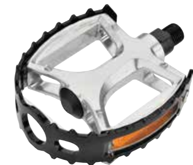
NWL-994 SIZE 111x93x24mm WEIGHT 450g/PR BODY Burnished silver alloy body CAGE Steel / Alloy AXLE Boron / Cr-Mo BEARING Loose balls REFLECTOR Included
