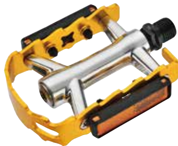
NWL-135B SIZE 103x62.5x24mm WEIGHT 250g/PR BODY Burnished silver alloy body CAGE Steel / Alloy AXLE Cr-Mo BEARING Sealed Bearing REFLECTOR Included
