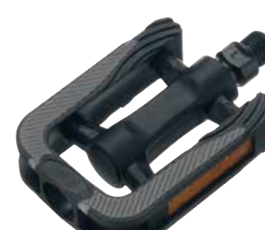
NW-410 SIZE 105x70x24mm WEIGHT 280g/PR BODY One piece PP body with TPR rubber AXLE Boron / Cr-Mo BEARING Loose balls REFLECTOR Included
