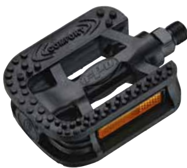
NW-352 SIZE 109x82x26mm WEIGHT 370g/PR BODY One piece PP body with TPR rubber AXLE Boron / Cr-Mo BEARING Loose balls REFLECTOR Included
