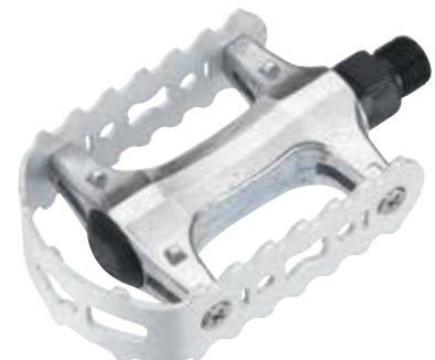
NWL-94K SIZE 101x63x24mm WEIGHT 353.5g/PR BODY Burnished silver alloy body CAGE Steel / Alloy AXLE Boron / Cr-Mo BEARING Loose balls
