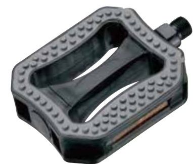
NW-350 SIZE 110x97x27mm WEIGHT 409g/PR BODY One piece PP body with TPR rubber AXLE Boron / Cr-Mo BEARING Loose balls REFLECTOR Included
