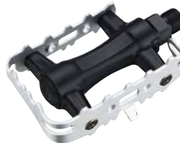
NW-91K SIZE 101x69x26mm WEIGHT 300g/PR BODY One piece PP body CAGE Steel ED / Alloy anodized AXLE Boron / Cr-Mo BEARING Loose balls TOE CLIP Available TOE STRAP Available
