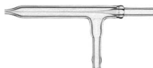
500-72 - C-Type Concentric Nebulizer, 1 lpm Ar, 30psi, 3mL/min
