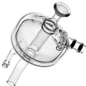
110-55J - Cyclonic Spray Chamber, Water-Cooled, 10mm Drain
