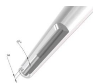
EZSS=3度斜角超細型(3mm) EZSS=3° SlimSuper(3mm)
