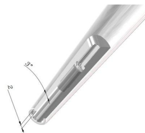
EZSUB=3度斜角極細型附螺絲 EZSUB=3° SlimUltra with back up screw
