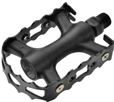
NW-499 SIZE WEIGHT BODY CAGE AXLE BEARING 109x63x22.5mm Alloy cage 320g/PR Steel cage 385g/PR One piece PP body Steel / Alloy Boron / Cr-Mo Loose balls
