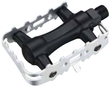
NW-91K SIZE WEIGHT BODY CAGE AXLE BEARING TOE CLIP TOE STRAP 101x69x26mm 355g/PR One piece PP body Steel ED / Alloy anodized Boron / Cr-Mo Loose balls Available Available
