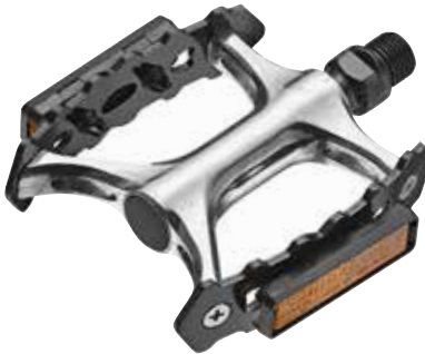
NWL-452L SIZE WEIGHT BODY CAGE AXLE BEARING 117x82x21mm 300g/PR Burnished silver alloy body Steel / Alloy Boron / Cr-Mo Loose balls
