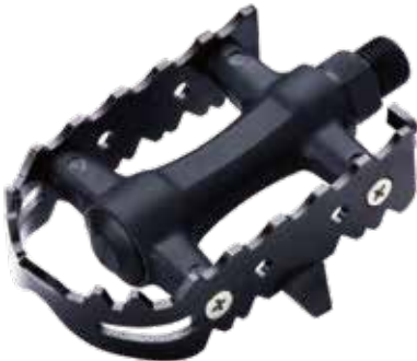
NW-93K SIZE WEIGHT BODY CAGE AXLE BEARING TOE CLIP TOE STRAP 110x62.5x25mm 415g/PR One piece PP body Steel Boron / Cr-Mo Loose balls Available Available
