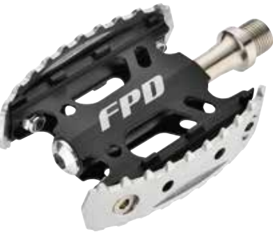
NWL-402BX SIZE WEIGHT BODY CAGE AXLE BEARING 102.8x77.1x27mm 320g/PR CNC alloy body Steel Cr-Mo Sealed bearing.
