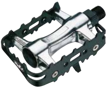
NWL-91K SIZE WEIGHT BODY CAGE AXLE BEARING TOE CLIP TOE STRAP 102x62x24mm 422g/PR Burnished silver alloy body Steel / Alloy Boron / Cr-Mo Loose balls Available Available
