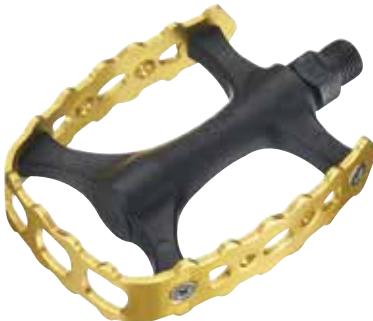
NW-99K SIZE WEIGHT BODY CAGE AXLE BEARING 110x82x23mm 288g/PR One piece PP body Steel / Alloy Boron / Cr-Mo Loose balls
