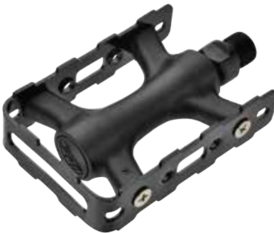
NW-517 SIZE WEIGHT BODY CAGE AXLE BEARING 96.4x62x24mm Alloy cage 264g/PR Steel cage 334g/PR One piece PP body Steel / Alloy Boron / Cr-Mo Loose balls
