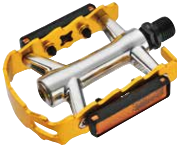
NWL-135B SIZE WEIGHT BODY CAGE AXLE BEARING REFLECTOR 103x62.5x24mm 250g/PR Burnished silver alloy body Steel / Alloy Cr-Mo Sealed Bearing Included
