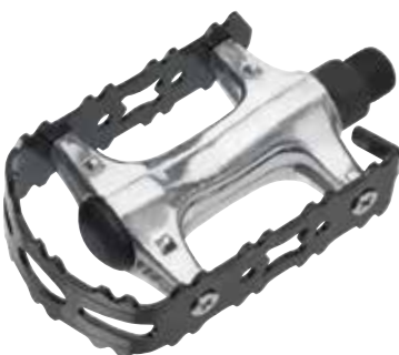
NWL-96K SIZE WEIGHT BODY CAGE AXLE BEARING 105x62x24mm 454g/PR Burnished silver alloy body Steel / Alloy Boron / Cr-Mo Loose balls
