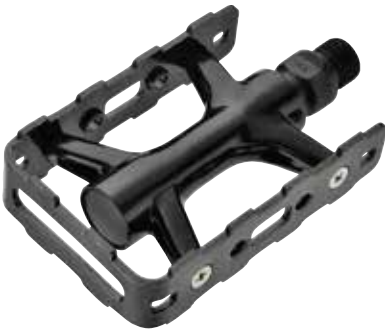
NWL-517 SIZE WEIGHT BODY CAGE AXLE BEARING 96.4x62x24mm Alloy cage 300g/PR Steel cage 370g/PR Burnished silver alloy body Steel / Alloy Boron / Cr-Mo Loose balls
