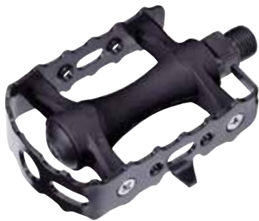
NW-90R SIZE WEIGHT BODY CAGE AXLE BEARING TOE CLIP TOE STRAP 106x62x25mm 410g/PR One piece PP body Steel / Alloy Boron / Cr-Mo Loose balls Available Available
