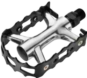
NWL-499 SIZE WEIGHT BODY CAGE AXLE BEARING 109x63x20mm Alloy cage 318g/PR Steel cage 358g/PR Burnished silver alloy body Steel / Alloy Boron / Cr-Mo Loose balls
