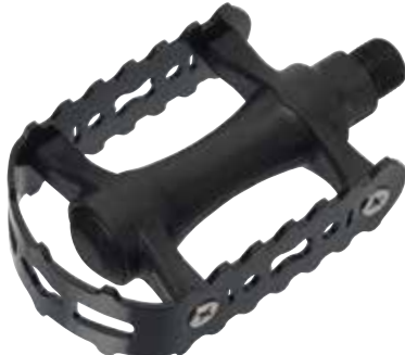
NW-94K SIZE WEIGHT BODY CAGE AXLE BEARING 101x62x25mm 288g/PR One piece PP body Steel / Alloy Boron / Cr-Mo Loose balls
